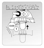
Remove gear tray from body by squeezing locator lugs one pair at a time lift corner.
