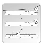
Fit water proofing power lead grommet (supplied) into selected body hole and puncture for powerlead. Blank off 'A' with 2nd grommet supplied if hole not used.
