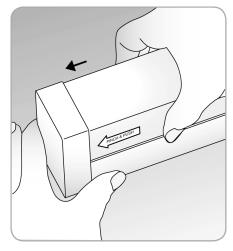
To remove the diffuser "pinch and push" the end marked with the arrow and push further into end. Pinch and push until the other end of the diffuser pops out.
