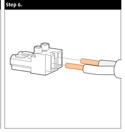
Pull powercable to female plug(f) & strip wires.
