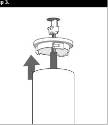
Feed powercable through opening of surface mounted disk(b).
