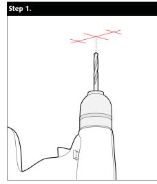
Mark ceiling and drill holes for powerfeed and pilot holes for fasteners if necessary.
