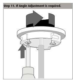
Rotate Surface mounted disk and re-fix mounting screws.
