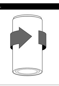
Insert 'can body'(a) into 'surface mounted disk'(b). Rotate 'can body'(a) anti clockwise to install.
