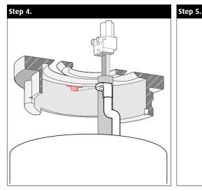
Insert lanyard into opening of surface mounted  $\mathsf{disk}(\mathsf{b}).$
