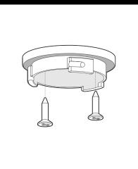
Fix surface mounted disk(b) to ceiling with screws.
