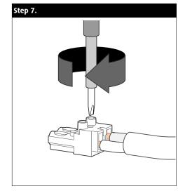
Insert stripped powercable into supplied plug(f) Connect plugs. and teriminate with flat screwdriver.
