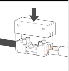
Insert supplied plug cap(g) over join.
