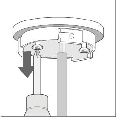
Back off screws installing surface mounted disk.
