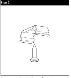
Fix mounting bracket(i) to ceiling with screws(k).
